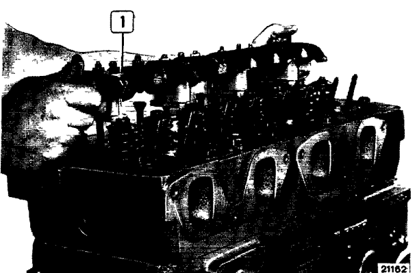
Remove the complete rocker carrier shaft (1)
