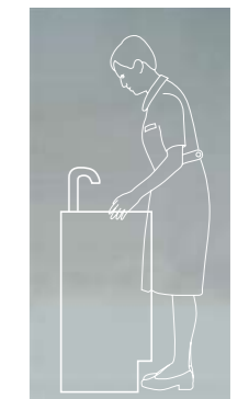
The sink is too low
